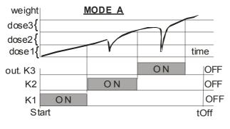
The start by active level of input Zero/Start at power supplying must be assessed according to the option 'taring at start'. If the option is active or inputs Zero/Start and Tare are united, you can use an impulse, not a constant input signal to avoid second taring at loss and second appearing of the power supplying voltage.
